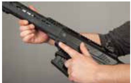
Photo 6 -) Push pivot pin at the front sight of lower frame by a tool or your finger as in the photo.
