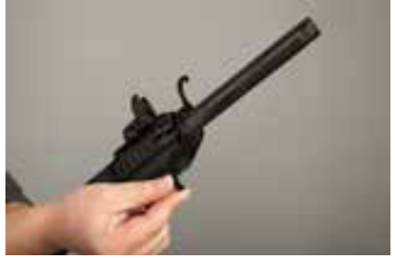
Photo 8 -) Use your AR12 Special Wrench Set for starting to disassemble forend of your shotgun.
